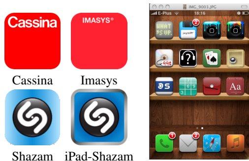
Figure 8. Icon boundaries. (left) Often icons differ only in regions close to their boundary. A good descriptor should hence consider the entire icon without reducing the importance of boundary pixels, as is done in SIFT. (right) Frequently, various visual symbols are attached to one of the icon’s corner, hence, the corner regions should be excluded from the icon descriptor.
