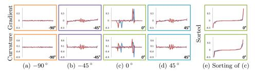
**Fig. 4. Gradients and Curvatures:** The resulting gradients and curvatures of the four curves in Figure 3 (a-d). While offering an improvement in terms of robustness to illumination differences, this representation is still sensitive to geometric distortions (c). By applying a sorting permutation, robustness to such distortions is enforced (e).
