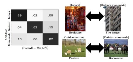
Fig. 8.  $1^{st}$  level confusion matrix: *Left:* The confusion matrix of our OTC descriptor on the  $1^{st}$  level of the SUN397 dataset shows that most misclassifications occur between indoor & outdoor man-made scenes, and within the two types of outdoor scenes. *Right:* Images in which the classification was mistakingly swapped.
