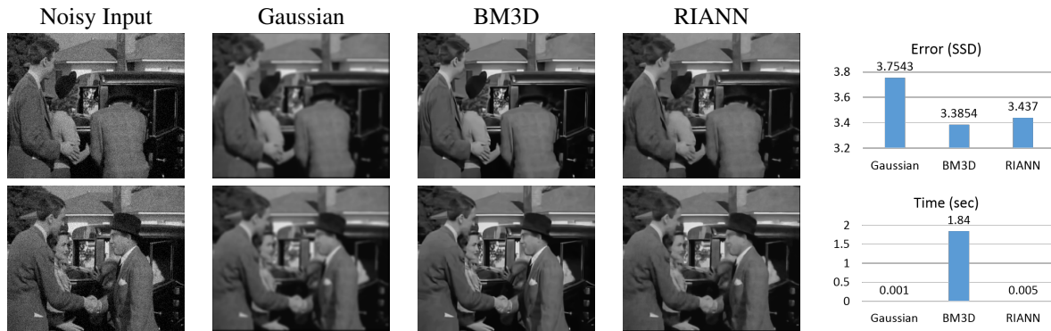
Figure 8. Denoising: The images are of two example noisy frames and their denoised versions obtained by Gaussian filter, BM3D, and RIANN. The charts compare run-time (per frame) and Sum of Squared Differences (per pixel) averaged over our test set. RIANN is almost as fast as Gaussian filtering while being only slightly less accurate than BM3D.
