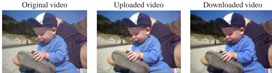
Figure 3. Degradation in quality. Uploading and downloading videos degrades their quality significantly and modifies colors. The main degradation in quality occurs at the upload process as can be seen by comparing the original frame on the left with the corresponding screen capture of the uploaded video in the middle. The download process introduces further degradation.
