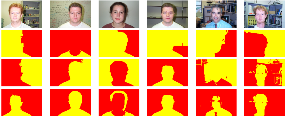
Figure 7. Image collection. Six examples out of a collection of 30 images of 5 different people. Top: Original images. Second row: Ncut segmentation. Third row: Our approach segmenting each image independently. Bottom: Our result with part sharing provides higher quality segmentation. See also Fig. 8
