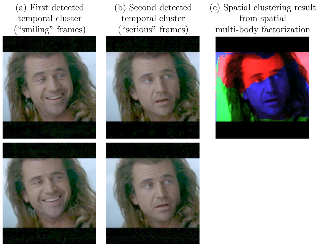
Figure 9. Temporal vs. spatial clustering using dense optical flow. Results of factorization applied to a sequence taken from the movie "Brave Heart". The actor (Mel Gibson) is serious at first and then smiles while moving his head independently from his expression throughout the sequence. Optical flow was estimated relative to the first frame and the clustering was applied directly to it. We set the number of clusters to 2 for temporal factorization and to 3 for spatial factorization. (a) Sample frames from the first detected temporal cluster, all of which show the actor smiling. (b) Sample frames from the second detected temporal cluster which show the actor serious. (c) Since optical flow was used, we could obtain dense spatial segmentation. This separated between the forehead, the mouth region and a dangling group of hair. These correspond to three independent motions in the sequence: Along the sequence the actor raises his eyebrows and wrinkles his forehead. Independently of that the mouth region deforms when the actor smiles. The group of hair dangles as the head moves, again independently from the other two motions (the motion of the hair at the lower left part of the image can be seen in the frames in (a) and (b)). Video can be found at http://www.vision.caltech.edu/lihi/Demos/TemporalFactorization.html
